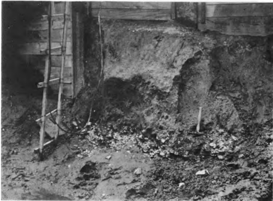
2. 縄文海進の高海面期を示す \pm 0 \sim \pm 3 m の海成層上限（尼崎市栗山） Outcrop of marine clay layer (Ma 13) showing marine limit at the high sea level of Jōmor Transgression.
